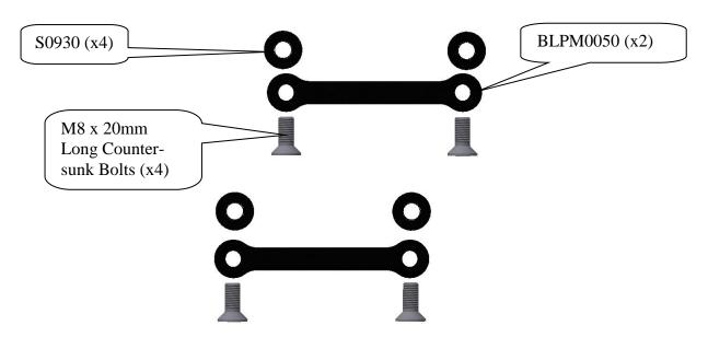
Please note that in cases where kits are packed with rubber washers holding the components onto the bolt – the rubber washers should be thrown away!
